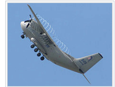
C-27J Spartan with propeller tip vortices condensation. The C-27J uses the same engines as the MV-22, but has higher disk loading.
