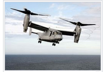
The MV-22 Osprey tiltrotor has a relatively high disk loading, producing visible blade tip vortices from condensation of the marine air in this photo of a vertical takeoff.
