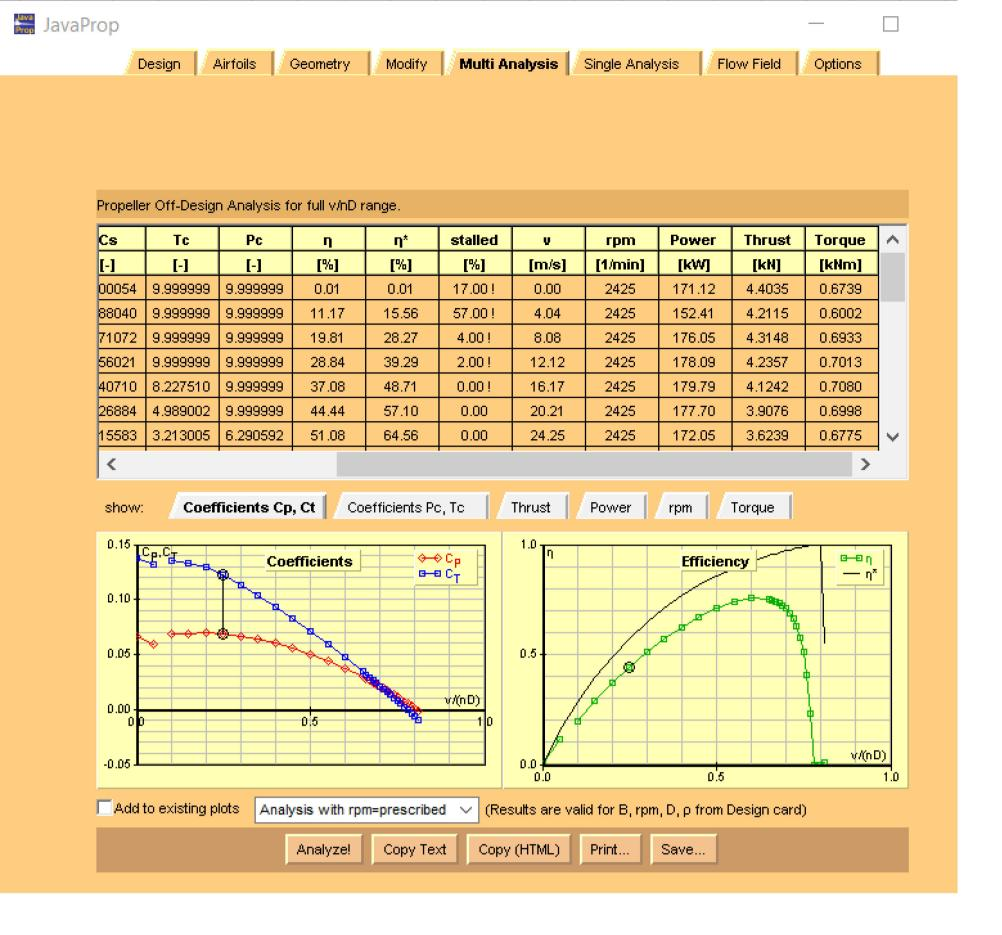
Propeller Static Thrust = 4.4035 kN 4.4035x6= 26.421 kN
