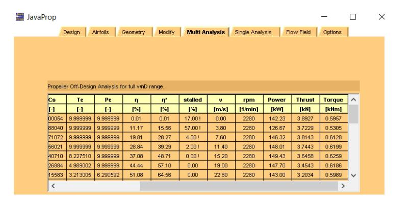
Drone wt (all sources) = 5700 lbs = 23.35 kN23.35 kN/6 = 3.89 kN needed per prop
