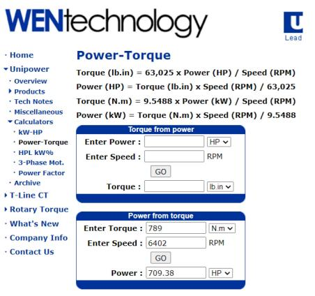
Thus to fly upward at a steady + vertical velocity of 17 ft/sec needs 709.38 HP per jet
