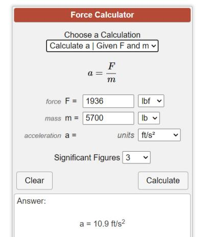
Thus the drone can be accelerated from 40 mph to 60 mph using 1936 lbs of  $\rightarrow$  directed force. This results in an  $\rightarrow$  directed acceleration of 10.9 ft/sec<sup>2</sup>
