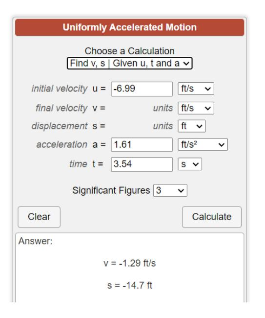
Thus while going from an airspeed of 30 mph to an airspeed of 40 mph, the drone went vertically \( \psi \) by 14.7 feet and its \( \psi \) directed velocity went from 6.99 ft/sec \( \psi \) to 1.29 ft/sec \( \psi \)
