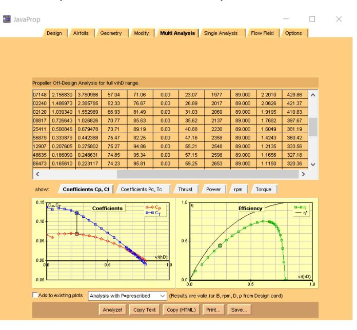
From JavaProp 55.21 m/s 2548 rpm 89 kW 1.21 kN 333.56 Nm 2548 rpm = mach 0.783
