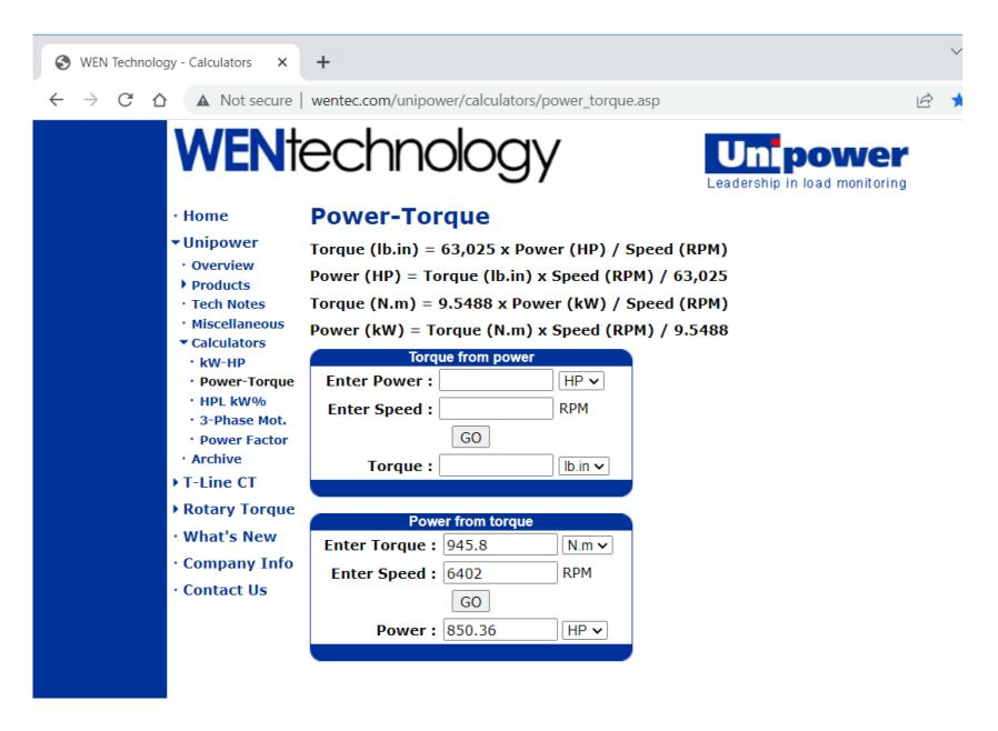
945.8 Nm running at 6402 rpm gives power of 850.36 HP (per engine), and 1701 total HP (for both engines)
