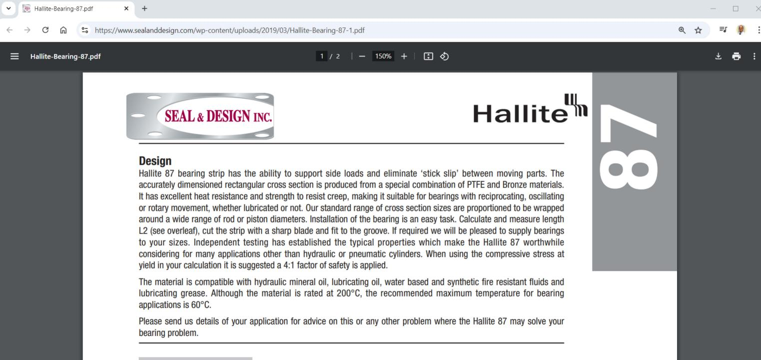
The material is compatible with hydraulic mineral oil, lubricating oil, water based and synthetic fire resistant fluids and lubricating grease. Although the material is rated at 200°C, the recommended maximum temperature for bearing applications is 60°C.
